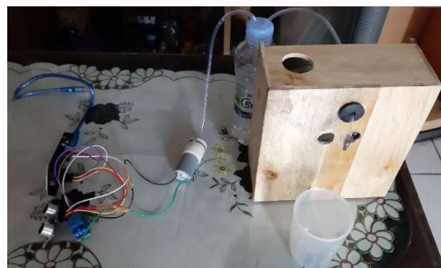
Gambar 9. Pengujian Rancangan Hand Sanitizer Otomatis
