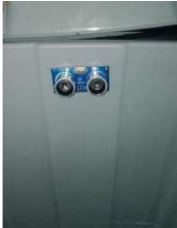
Gambar 6. Instalasi Sensor HC-SR04
