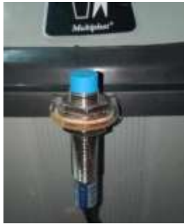
Gambar 8. Instalasi Sensor Induktif Proximity
