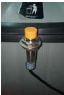
Gambar 7. Instalasi Sensor Kapasitif Proximity
